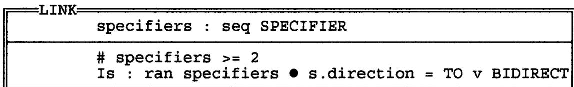
Figure 3. Z Notation Specification of a Link
